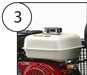
3 Fill with fresh, regular unleaded gasoline with a minimum of 87 octane. Leave a 1-inch air gap between fuel and cap.
