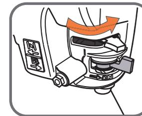
7 Ensure Choke is Completely Open During Operation
