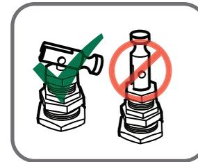
1 Leave unloader valve toggle down AT ALL TIMES
