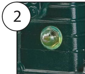
2 Most ROLAIR® compressors come pre-filled with oil. Check oil sightglass before starting and add if necessary. See manual for fill amount and oil specifications.
